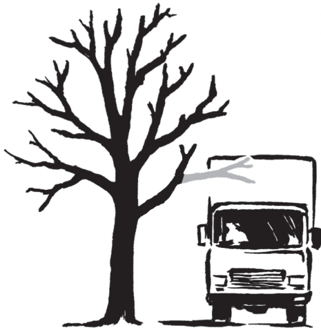
Correct clearance cutting for branches over 10 cm in diameter (cutting as far as a supplying branch)
